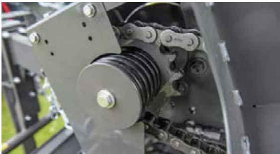
The free wheel sprocket ensures that the drive train is protected against damage in the event of a rotor blockage.
