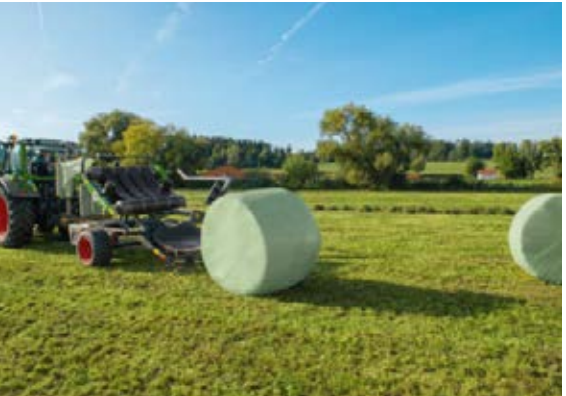
The Rollector 160 is equipped with a bale unloading table with active drop – this effectively avoids damage to the film.
