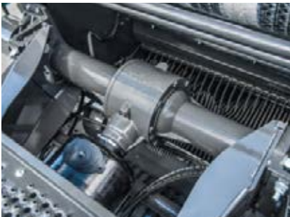
The Power Split gearbox runs at a PTO speed of 540 rpm.
