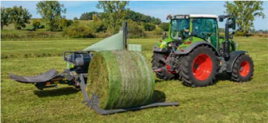
Both the loading arm and the wrapping table can be adapted to different bale sizes. Safely pick up bales with a diameter of 1.25 m to 1.6 m and pack them airtight in film.
