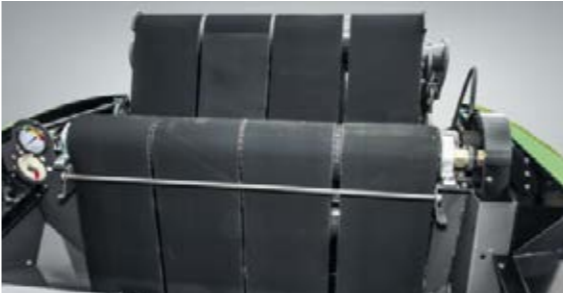
Four symmetrically arranged infinite belts shape the bales. The drive is powered by two drive rollers to transfer just the right force.
