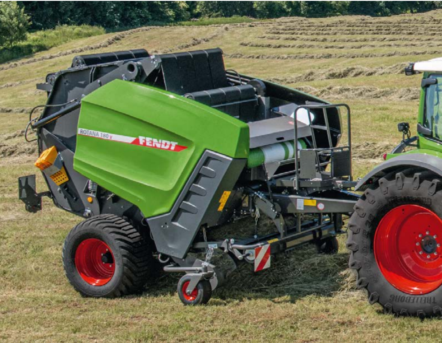
The uncontrolled pick-up is both maintenance-friendly and smooth-running. The gauge wheels are fixed or rotatable depending on the configuration.
