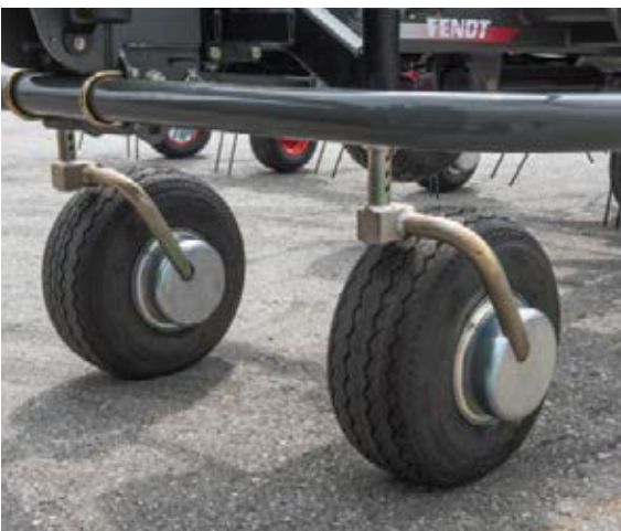
□ The optional mobile feeler wheels optimise the ground tracking, and ensure clean raking and sward protection. (Fendt Twister 901 T)
